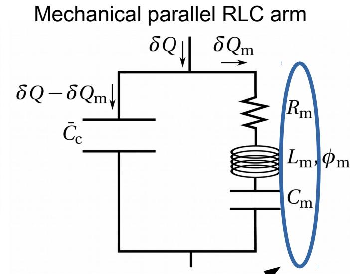
Mechanical equivalent circuit parameters
