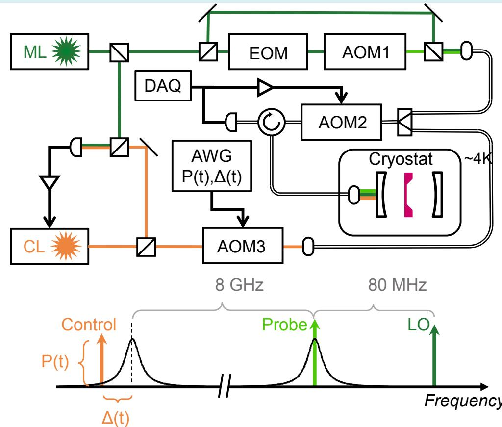
The membrane motion of one mode modulates the intracavity field, which drives the other mechanical mode, and vice versa.
