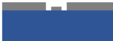
d) Spin PMMA, EBL, Etch the gate region
